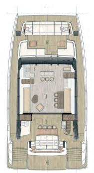
4/ 300 m<sup>2</sup> (3,230 sq ft) of deck area, 80 m<sup>2</sup> (860 sq ft) for the flybridge and 100 m<sup>2</sup> (1,076 sq ft) of cabin space in the hulls: this supercat is competing with luxurious monohull superyachts of at least 35 m (110') in length.
